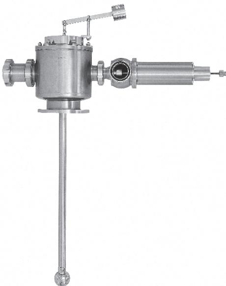
Tanks or containers are often equipped with a combined CIP/gas tank line. This ends at the tank in a cleaning air/valve combination (RLV combination) equipped with a tank connection. This compact multifunctional unit controls the supply of CIP fluids or the supply and removal of the gas flows / CO<sub>2</sub> via an integrated switching valve. This guarantees safe media management.
