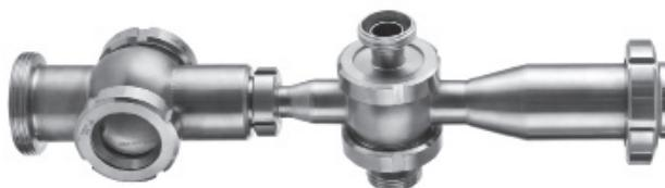
The VARIOair aeration armature is predominantly used in yeast and wort aeration in breweries. The dissolved oxygen increases the yeast growth and consequently later in the fermentation phase the sugar breakdown and the alcohol formation. The armature can also be integrated as an aeration unit in other industry branches.
