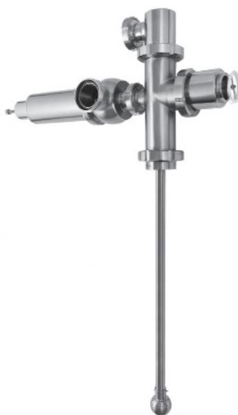
Tanks or containers are often equipped with a combined CIP/gas tank line. This ends at the tank in a cleaning air/value combination (RLV combination) equipped with a tank connection. This compact multifunctional unit controls the supply of CIP fluids or the supply and removal of the gas flows / CO<sub>2</sub> via an integrated switching valve. This guarantees safe media management.
