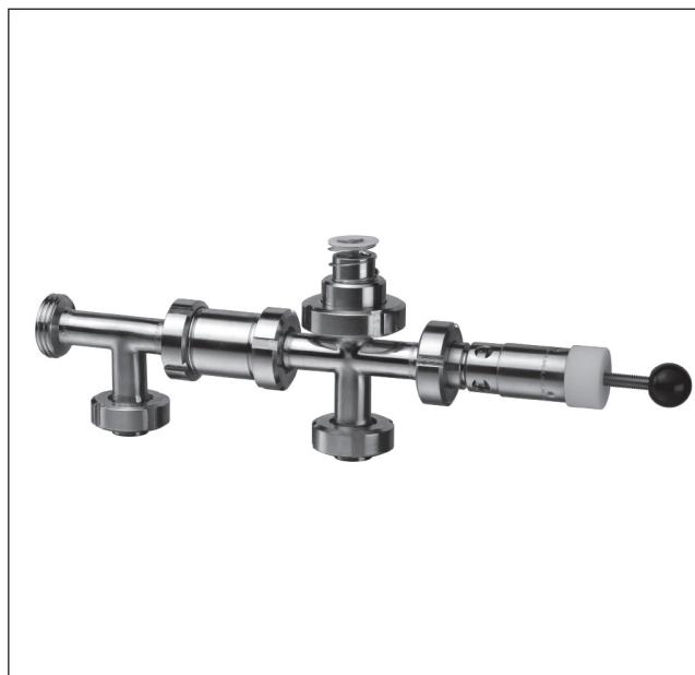
Tanks or containers are often equipped with a combined CIP/gas tank line. This ends at the tank in a cleaning air/valve combination (RLV combination) equipped with two tank connections. This compact multifunctional unit controls the supply of CIP fluids or the supply and removal of the gas flows / CO<sub>2</sub> via an integrated switching valve. This guarantees safe media management.
